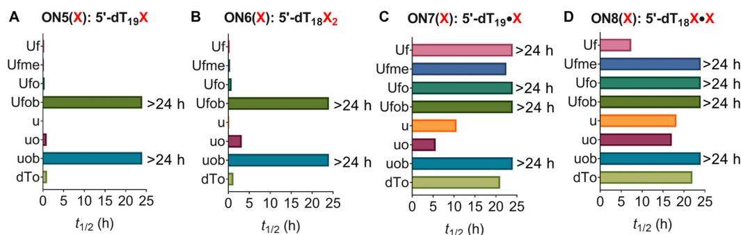
**Figure 2.** Relative stabilities toward 3'-specific exonuclease degradation. ONs (0.1 mg/ml) with (A, B) or without (C, D) additional PS modification (●) were incubated with SVPD (150 mU/ml) in 50 mM Tris (pH 7.2) buffer supplemented with 10 mM MgCl<sub>2</sub> and monitored via IEX-HPLC. Decay curves used to calculate half-lives  $t_{1/2}$  [h] are shown in Supplementary Figure S1 (Supplementary Materials). Values for Uf/Ufo/Ufob are from ref. 16.
