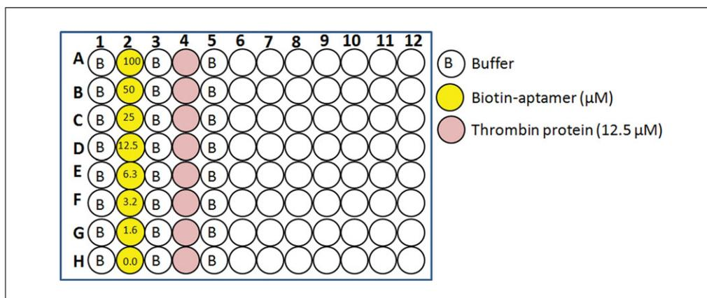
**Figure 7.25.4** Plate map diagram for optimization of aptamer loading on the streptavidin biosensors.
