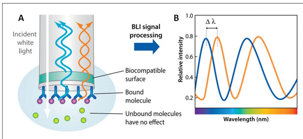
**Figure 7.25.1** The principle of biolayer interferometry (BLI). **(A)** Schematic drawing of the light interference on a biomolecule-bound layer and an internal reference layer of a fiber-optic biosensor. **(B)** The wavelength shift of the interference pattern caused by the target binding is measured in real time (provided by Dr. Sriram Kumaraswamy and Dr. Gemma Milan from FortéBIO, a division of Pall Life Sciences).
