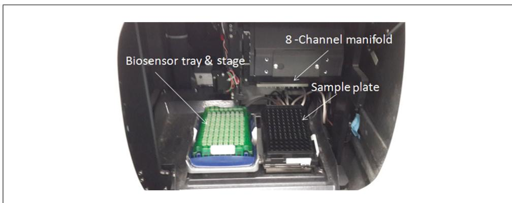
**Figure 7.25.6** The internal layout of the Octet System consists of a biosensor stage (left position) and a sample microplate stage (right position). The eight-channel optical manifold can acquire up to eight biosensors for parallel processing.
