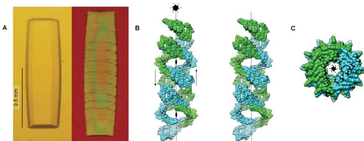
**Fig. 2** (A) Native homo-DNA crystal (left) and a crystal displaying a left-handed helical fracture (right). (B) Stereo diagram of the *left-handed* double-stranded superhelix formed around *right-handed* sixfold screw axes ( $6_1$ ). (C) The superhelix viewed along the screw axis. Green and cyan duplexes are symmetry-related through local dyads (two of which are shown in the figure). Green duplexes among themselves and cyan duplexes among themselves are related *via* the sixfold screw axis.
